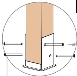
Make sure to first cut your wood post down to 84," this is a critical step. With the six bolt down brackets installed plumb, proceed to set the 4x4x10' (10x10x300cm) wood posts in place. Secure the wood posts using the screws provided with the bolt down bracket kit. Repeat for all wood posts.
