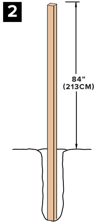
2 After holes are dug and cleaned, place the 4x4 (10cmx10cm) wood post into a hole ensuring it's level and square to string lines. The final post height should be 84" (213cm) out of the ground. If a post is higher because of obstructed excavation of footings, please cut down the height accordingly.
