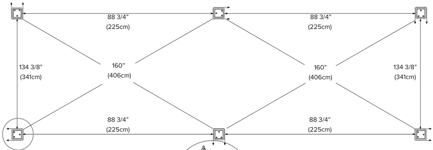
Orientate brackets accordingly to reduce offset motion of posts. (direction of arrows denote flange opening)
