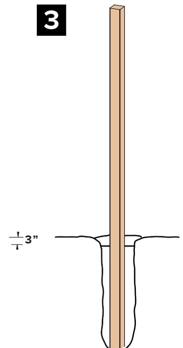
3 Fill the vacant hole with pre-mixed concrete all the way to within 3" (7.6 cm) of the top of the hole. Once concrete has set, backfill and compact the 3" (7.6 cm) space with soil.
