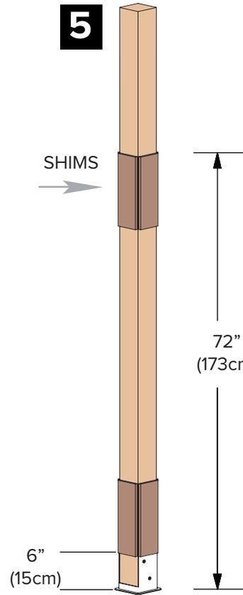
In order to create a snug fit between the wood posts and the inner cavity of the vinyl posts, it will be necessary to "build out" the 4"x4" (10cmx10cm) posts near the bottom and the top using 1/2" x 3 1/2" x 12" (1.27x 8.89x365cm) shims. Follow instructions as illustrated.
