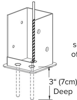
Proceed to install three 2 3/4" (6.985cm) concrete screws into the bottom base of the bolt down bracket (Not included).
