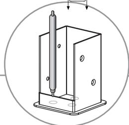
You can mark out the location of bolt down brackets accordingly using the base of the bracket if desired.
