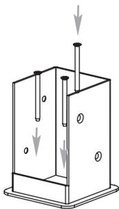
Using a 3/16" (0.47625cm) masonry drill bit (not included), drill 3" (7cm) deep holes to allow installation of 2 3/4" (6.985cm) concrete screws (Not included).
